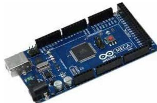
Figure 6: The Arduino Mega
