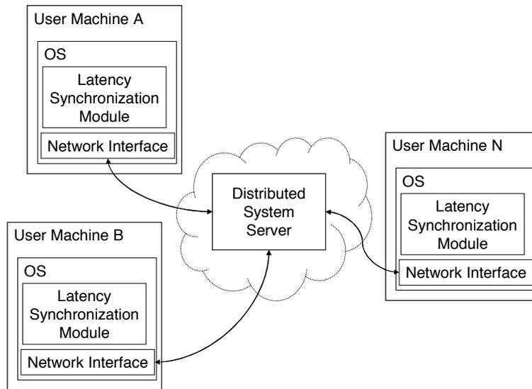
**Figure 1. System Diagram of the Latency Synchronization System**
