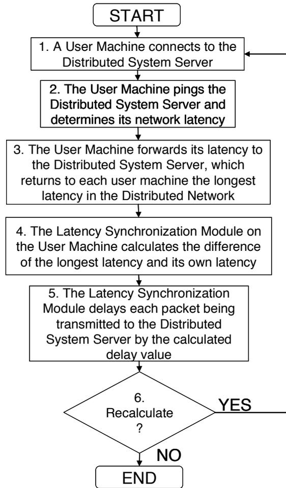
**Figure 2. Method for synchronizing latency using Latency Synchronization Module**
